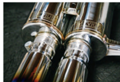
Note the quality of the welds. The MXP system uses four straight-through mufflers rather than a large single unit to save weight while still producing an aggressive yet street-friendly tone.
