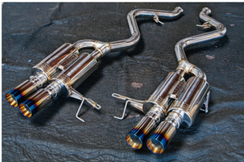
The beautiful Mackin Extreme Products (MXP) Mevius stainless steel rear exhaust section uses the stock hangers for a factory fit.
