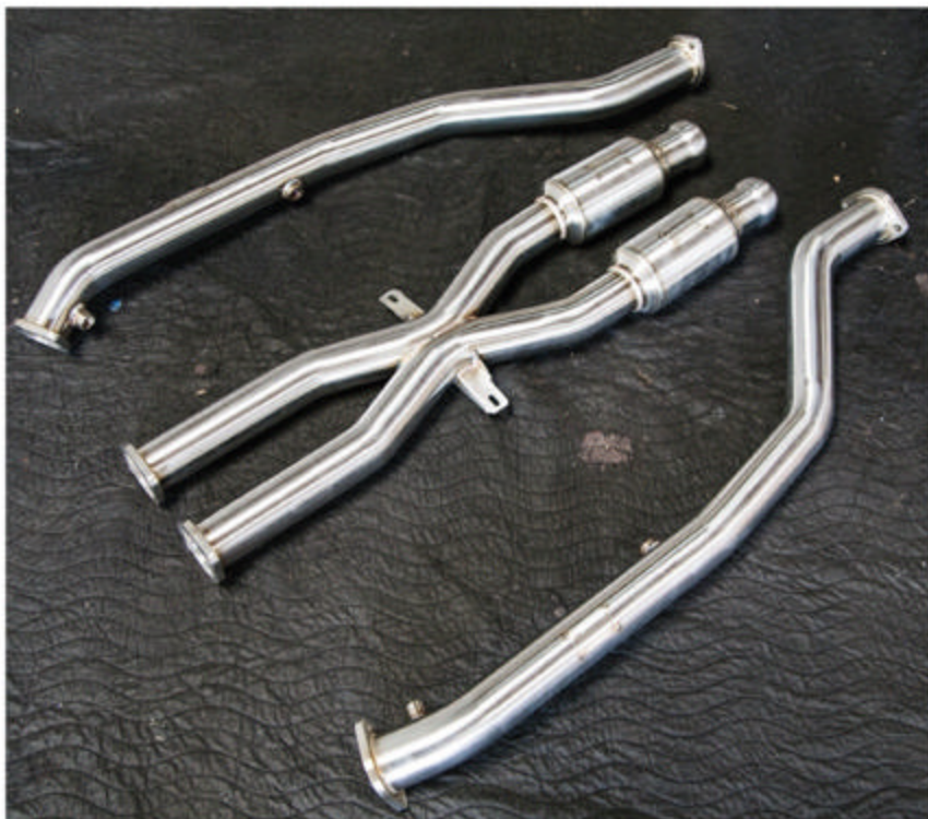
The entire Macht Schnell stainless steel race X-pipe system bolts into place using stock mounting hardware.
