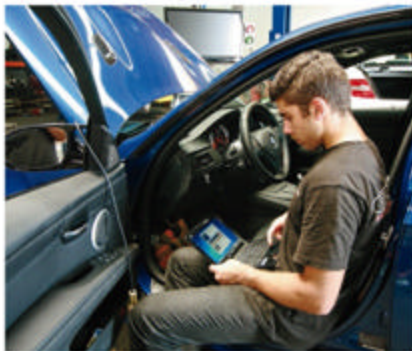
Adam uploads the ESS Tuning custom naturally aspirated 91-octane tune. Should we make changes that necessitate a re-tune, the provided OBDII port connector and cable make it easy to get tunes from ESS via email.
