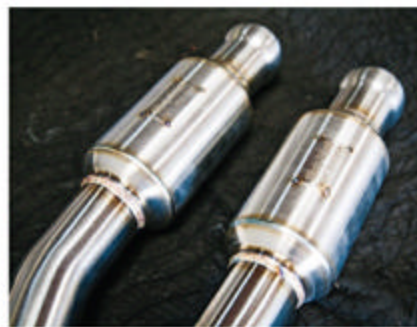
There's nothing worse than a droning exhaust system. Macht Schnell includes a pair of resonators in its X-pipe to help cut drone and lower decibel levels without hindering horsepower.
