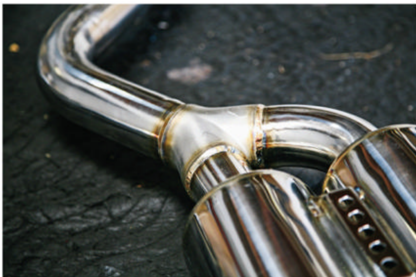
High-quality merges help preserve flow for increased power and a crisp sound. The MXP system is an octave higher than other systems, giving it a supercar tone more akin to a V-8-powered Ferrari under WOT.
